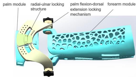
Fig. 1: Overall mechanism of the protective gear.
