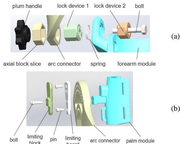
Fig. 2: (a) Palm flexion-dorsal extension locking mechanism
