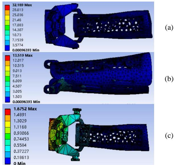
Fig. 7: (a) Equivalent stress nephogram of whole module
